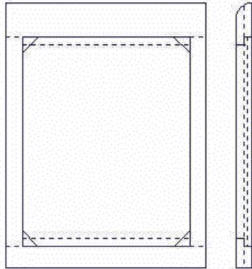
**Figure III (above):** When the ground glass eventually is installed two pieces of 0.8 mm brass shim are placed between the birch plywood and the ground glass so that the focusing surface of the ground glass is 4.8 mm from the bottom surface of the ground glass frame. The ANSI standard has a plus minus tolerance of 0.18 mm. Use a pair of Vernier calipers or a micrometer to check the measurements.
