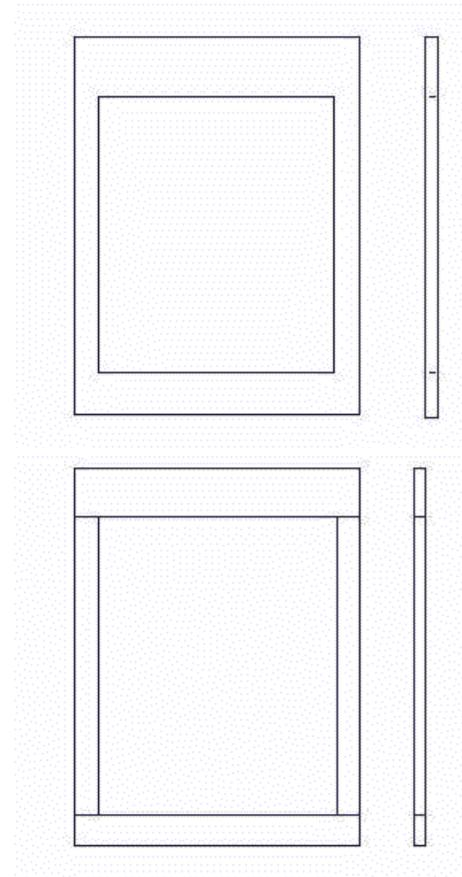
**Figure II (above):** Pieces of 5 or 6 mm hardwood strip are cut to form a frame which is glued on top of the
