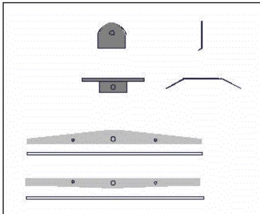
**Figure VI :** The drawing shows the pieces of brass from above and in profile. The bottom piece is bent to form a spring which exerts a certain pressure on the ground glass. The top piece is bent about 60–70 degrees.
