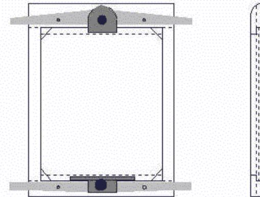
**Figure V (above):** The mechanism which holds the ground glass in place is made of 1 mm brass. (See Figure VI.) A hole is drilled in both pieces. There will be a screw from underneath the ground glass frame
