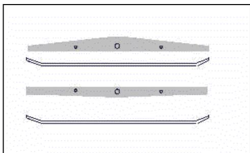
**Figure VII:** The ends of the brass strips are bent upwards to keep the leaf spring in place.
