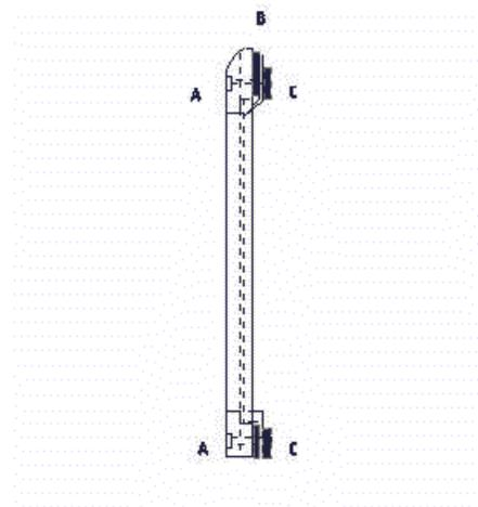
**Figure VIII:** The brass strips (B) and the ground glass retaining mechanism are held in place by screws (A) from underneath the ground glass frame. Knurled nuts (thumb nuts) (C) are used for fastening.
