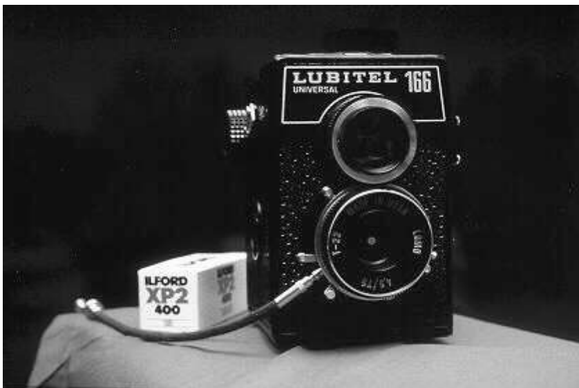
A Lubitel 166 modified for pinhole photography
